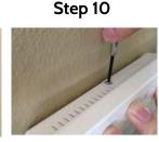
Replace retainer screw and tighten
