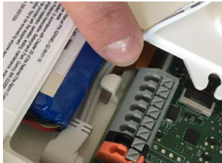
Route the wire behind the retainer clip
