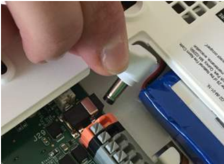
Plug in the power connector
