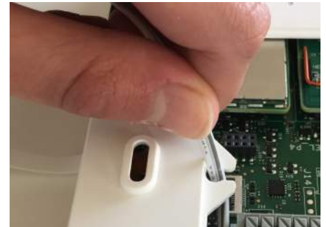
Insert the wire into the strain-relief
