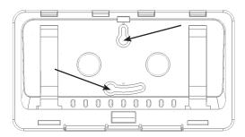
The power cable can exit the enclosure through the rectangular hole (typical) or can be completely hidden by drilling a third (big) hole in the wall inside one of the big round holes in the plastic. This will require fishing the wire behind the drywall to a location with an AC power outlet. Regardless, during reassembly, be sure to use strain relief channels for the power cable. Details on this are found on the "More Tips" page of this document.
