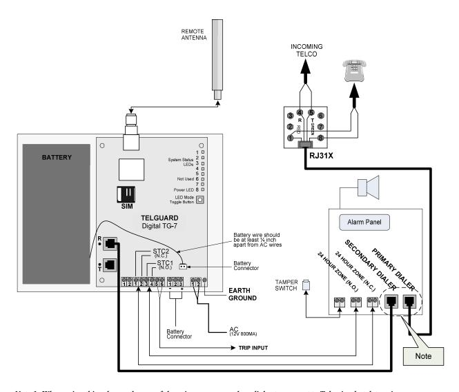
Note 1: When using this scheme, the use of the primary or secondary dialer to connect to Telco is what determines whether the TG-7 is meant to work as a back-up or primary communicator.
