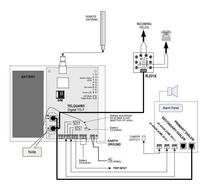
Note: When using this scheme, the programming of the TG-7 is what determines whether the TG-7 is meant to work as a back-up or primary communicator.
