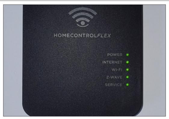
The FlexHub Z-Wave Controller has five LED indicators as shown in the chart on the following page. A functional description for each LED is listed in the table.
