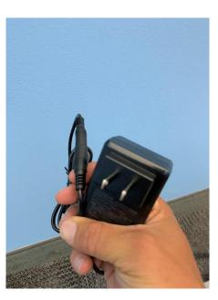
**Step 13**Connect the power supply (included with the scanner) to the DC12V extender cable at the base of the stand, and plug the power supply into the electrical source
