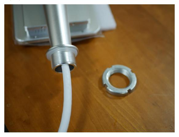
Step 5. Feed the cables from the device through the circular opening on the top of the stand. Be careful while doing this. You do not want the cables getting damaged during this process.
