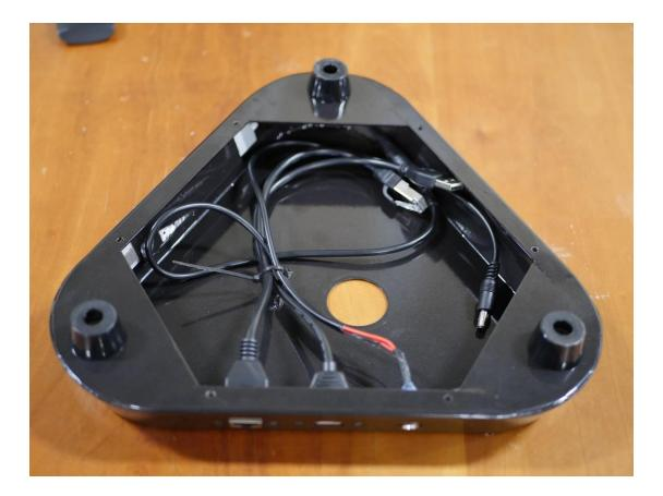
Step 4. Remove the locking threaded washer from the device. This piece ensures the device stays in place and is stable while attached to the stand.
