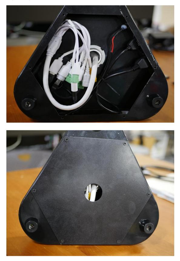
Step 8. Safely return the cables into the stand and attach the bottom plate.
