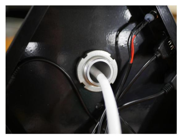
Step 7. Attach the three internal cables from the stand to their respected spot on the cable grouping coming from the device. Power will be attached to the 12V DC connection. The USB will be attached to the USB host cable and the ethernet cable (RJ45) will be attached to the RJ45 cable.
