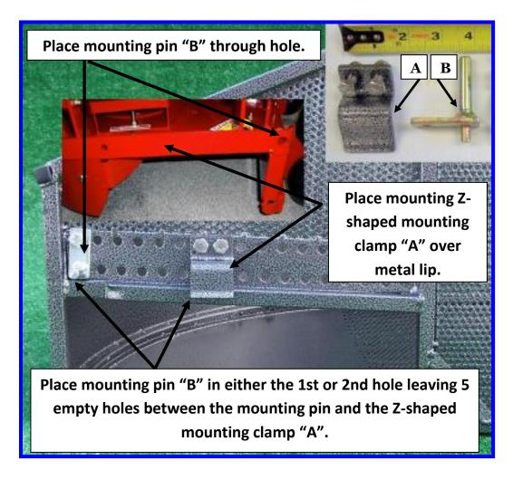
Bracket "A" should be bolted to the catcher towards the rear. Far enough back to clear the ears that hold the deflector, approximately hole 7 & 8. Bracket "A" slides down on the vertical piece of steel that the deflector ears are welded to.
