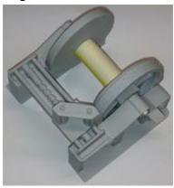
Step 5: Attach the cable guide arm with the ninth brass pin to the front (this may require a little boring of the holes as they can sometimes clog during the casting process, try using a small diameter nail or sewing needle to clear the hole). Now attach the entire front piece to the side pieces using CA Glue and the four provided screws. As shown in the following image:
