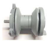
Step 9: Attach the cable guide arm with the ninth brass pin to the front (this may require a little boring of the holes as they can sometimes clog during the casting process, try using a small diameter nail or sewing needle to clear the hole). Now attach the entire front piece to the side pieces using CA Glue and the four provided screws.
