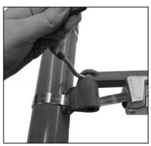
6. Pull cutting handle to cut the band. When applying Giant Band clamps, prior to cutting off clamp, release band gripper and push tool nose away from buckle approx. ¼".
