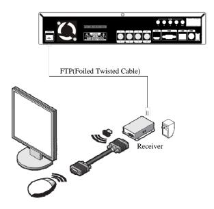
2. Because all the case has different cable length, you should adjust the GAIN and PHASE in Receiver to get a most proper VGA output. You can use the small cross screw driver for adjusting at the edge of Receiver.
