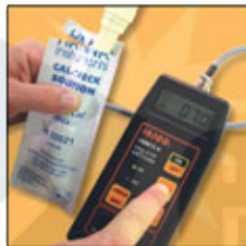
Press the "CHECK" key A green light indicates the meter is calibrated
