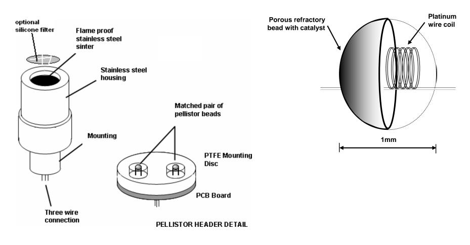
Combustible sensors detect gas by catalytic combustion
