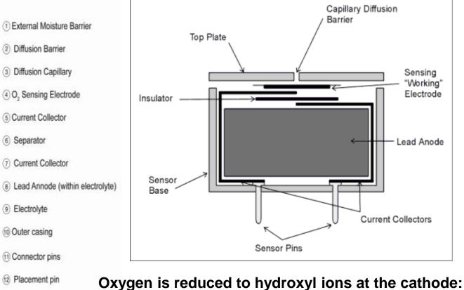
Oxygen is reduced to hydroxyr ions at the cathods  $O_2 + 2H_2O + 4e \rightarrow 4OH$ -Hydroxyl ions oxidize the (lead) anode:  $2Pb + 4OH \rightarrow 2PbO + 2H_2O + 4e$ -Overall cell reaction:  $2Pb + O_2 \rightarrow 2PbO$
