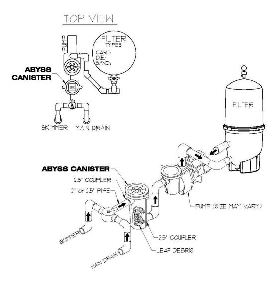
**CAUTION:** The Abyss canister must be plumbed between the pump and any suction side valves in order to prevent excessive water surges and pressures
