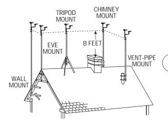
Follow the instructions supplied with the antenna mount and secure the mast to the mount.
