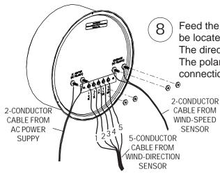
Feed the cables through the wall to where the read-out is going to be located. Attach the wires to the rear of the read-out as shown. The direction wires must follow in sequence for the direction sensor. The polarity does not matter for the wind speed or power supply connections. (Do NOT adjust the nuts that are already on the meter).
