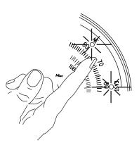
After setting the Gust Register turn the knob clockwise until the reset arm is parked near the six o'clock position. Failure to do so may damage your meter.
