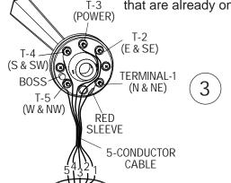
Feed the terminal lug end of the five-conductor cable through the other rubber boot and connect the lugs to the terminals on the bottom of the wind-direction sensor. (Do NOT adjust the nuts that are already on the sensor). The red sleeve indicates wire #1.
