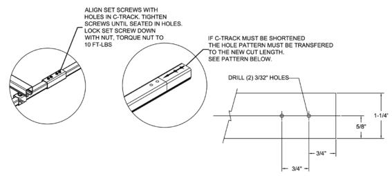
4.2.1 Track joints clamp for secure attachment and proper alignment of track section. Each kit includes four set screws and nuts. Welded splice assemblies are also available.
