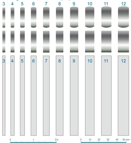
MEASURE THE ABOVE BAR TO ENSURE IT HAS PRINTED EXACTLY 2 INCHES OR 50MM, LONG. IF MEASUREMENT IS NOT ACCURATE, RING WIDTH MEASUREMENT WILL NOT BE COMPLETED PROPERLY
