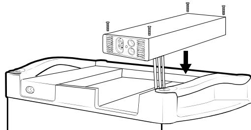
5. Gently set in the Solar Charging Optimization Module into place, tucking the cables into the opening.
