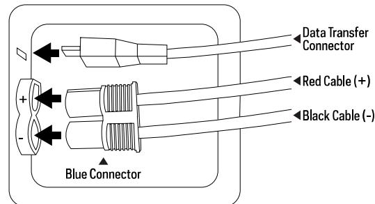
3. Take note of the positive and negative terminals on the Yeti's port, as well as on the blue connector. Insert the blue module connector into the module port on the Yeti Lithium, matching positive to positive, negative to negative.
