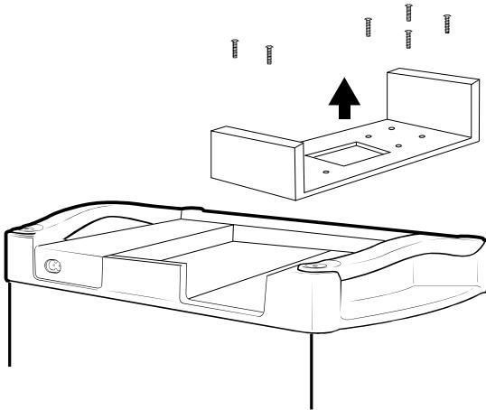
2. Open the lid of the Yeti Lithium and remove the expansion module carriage from the Yeti by removing the six screws and sliding out the carriage.
