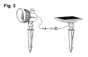
Note: 45 degree toward the south is the recommended angle and direction in North America to absorb maximum sun energy during the day.
