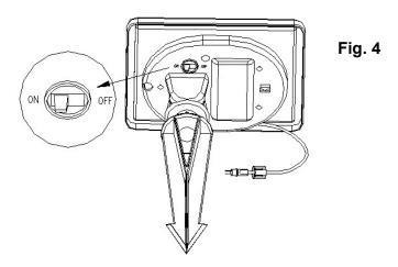
**NOTE**: For best results the solar spot light must be charged for two full sunny days while in the "ON" position.
