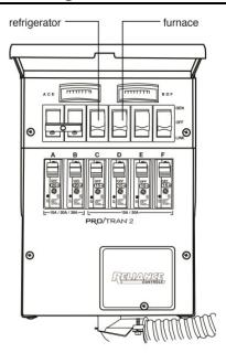
To maximize the efficiency of your generator, divide appliance circuits and others requiring higher wattage between adjacent circuit selector switches of the transfer switch so that a usage balance is achieved between the opposing legs of the generator power.
